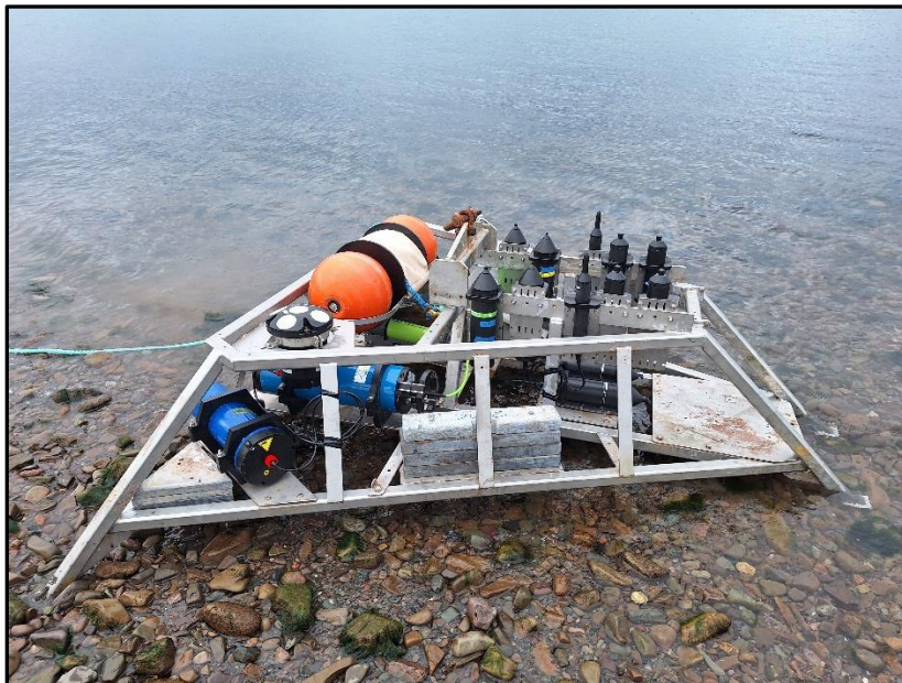
Figure 13: FAST-2 platform equipped with five Innovasea acoustic receiver technologies (with duplicates for redundancy), an ADCP and hydrophone for recording flow speed and underwater noise.
